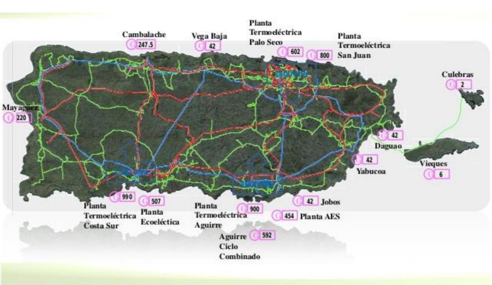
230 kV — 115 kV — 38 kV
