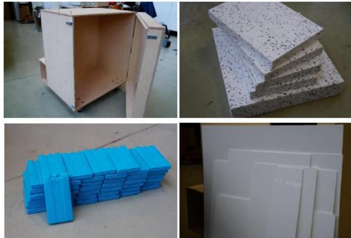
Figure 23: Wooden box (u.l.), polystyrene insulation material (u.r.), ice packs for ice storage around the evaporator (d.l.) and the acrylic glass plates for the internal covering
