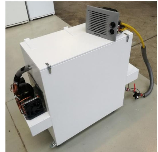
Example System 3: Water Chiller for cold rooms And water bath milk cooling
