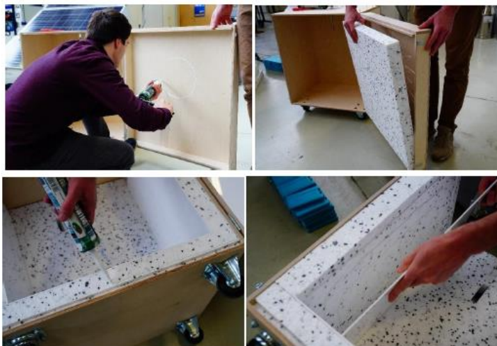
Figure 24: Gluing of the polystyrene insulation and internal acrylic glass covering
