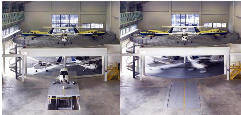
Schätz Vertical is the world's first rotating aircraft parking system measuring 22m in diameter and allows easy and safe handling of up to 14 aircraft on only 445 m<sup>2</sup> of land. The patented storage device saves land investment costs by 40% in addition to reducing delays, damages and high costs of manpower and operation while jockeying the aircraft.
